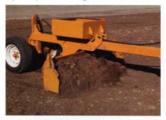
Optional Spill Guards allow this unit to double as a box scraper. The guards can easily be adjusted to the angle of the moldboard or flipped up, with the ease of spring loaded latches.
