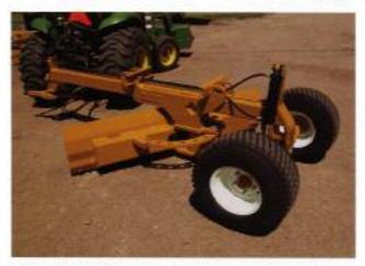
The trunnion style hitch, fastened to the tractor's 3-point arms, controls blade height, while providing superior maneuverability. The moldboard can be adjusted up to 45º left or right.
