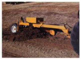
Heavy weight makes this a work horse for many jobs around the yard or construction job. A 3/8" thick moldboard and 1" plates on the frame give this compact size unit industrial strength.
