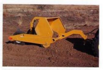
Material can be spread thin or stock piled, with full control of the bowl dump angle and blade height.
