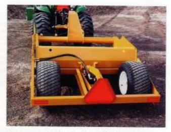
Narrow over-all width allows for working close to buildings or other obstructions. Large tires give flotation in soft soil.
