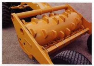
Cleaners are reversible, and will work forward or backward. Bungs are provided in both ends of the drum for filling with water or sand.
