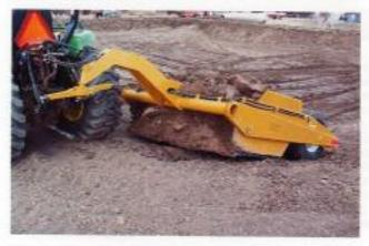
The trunnion style hitch and gooseneck frame provide for up to 90° turns, with 30° of oscillation, for exceptional agility on rough terrain.
