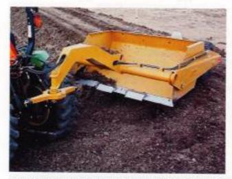
The "segmented frost bit" style blade increases penetration in hard soil, while maintaining a flat cut.
