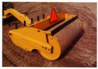
The steel roller on the RB-R model breaks clods, smooths, and packs. The drum can be filled with fluid or sand for added weight. It's mounted on sealed ball bearings.
