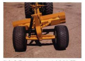
Hydraulic tilt gives on-the-go control of pitch, 20° up or down. Maintain a crown on your driveway, or shape your landscape to any contour. Large tires provide flotation and blade stability.
