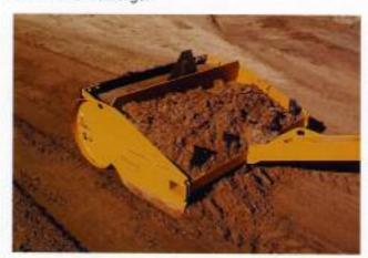
With more than 20" between the frame and moldboard, and adjustable side skirts to hold the load in, this unit provides exceptional capacity.
