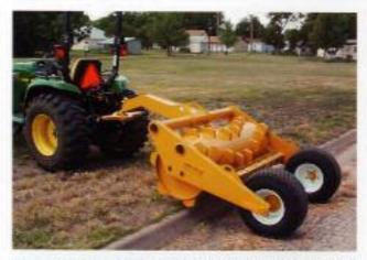
The drum can be raised while making sharp corners to prevent loosening the soil, and to allow travel over streets and sidewalks.
