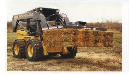
Using hydraulic muscle for bale handling is not limited to large machinery. Now you can do a big job with a little loader. This model helps dairy farms, horse ranches, landscapers, or construction crews with their hay or straw handling chores. The Model 50 will handle five bales, which is half of the Model 1000 accumulator's package. If you want to automate your hay handling, but don't have a large loader, or need the maneuverability of a skid-loader, this is your answer.
