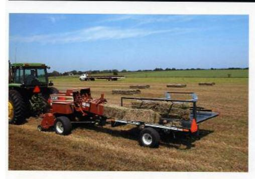
Towed behind the baler, the accumulator is powered by the tractor's hydraulic system. As the baler pushes the bales onto the accumulator, a pivoting arm automatically lifts two bales at a time and places them on the bed.
